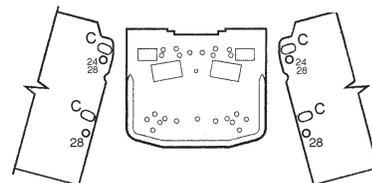
Attach the top rails to the vertical end cap using the hole patterns shown above using #10 x 1/2" screws. Example: On the ends of the pool, attach top rail hole "C" to vertical cap hole "21" and top rail hole "C" to vertical cap hole "24".
