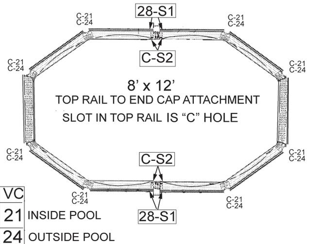
REFER TO THE DIAGRAM BELOW FOR TOP RAIL HOLE IDENTIFICATION
