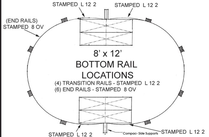
Place bottom rails stamped "L 12 2" on the outside of the side verticals. Place bottom rails stamped "8 OV" on the ends of the pool.
